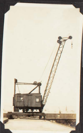
STOTHERT & PITT, 5-TON ROOF CRANES, TRAVERSE FULL WIDTH OF SHED ROOFS. MAX. RADIUS 3 FEET.
