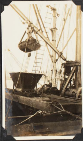
S.S. "KAITANGATA" DISCHARGING BY MEANS OF SMALL CRAB ON SHIP'S DECK TRIPPING INTO TRUCK ON TRAMLINE LAID OVER HULK, TRUCK HAS HINGED BOTTOM WHICH DROPS AT END OF LINE
